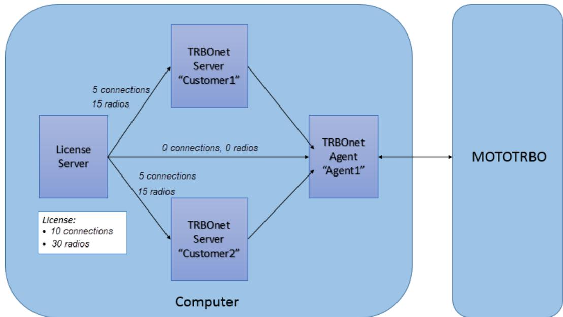
If you give 5 remote dispatch connections and 15 radios to one TRBOnet Server, the other TRBOnet Server can get the remaining remote dispatch connections and radios. TRBOnet Agent does not require any of these resources and should be configured to get "zero" values.
