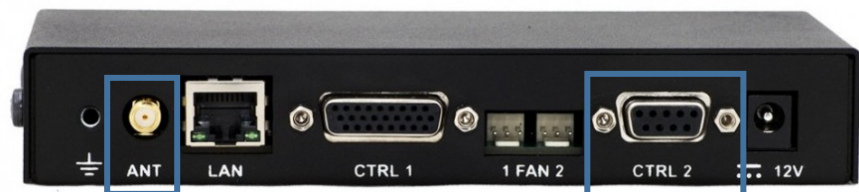
Figure 12: The antenna input and the CTRL2/DB9 connector of the IP controller
