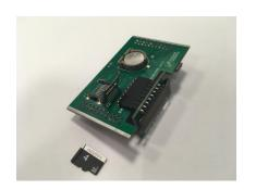
On the CPU board disconnected from the USB cable, use tweezers or a reliable short-wire jumper to short-circuit the two VIA-contacts located next to the battery.
