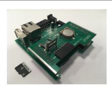
o Separate the CPU board from the GATE board.
