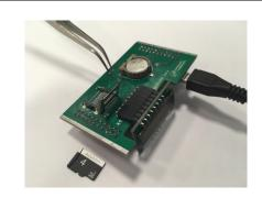
When connected via USB, the CPU board with the short-circuited contacts will be detected by the Device Manager and by Swift CPS as "STM32 Bootloader" or "STM Device in DFU Mode" (depending on the OS version).
