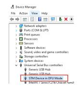
Once the device is detected by the PC as "STM32 Bootloader" or "STM Device in DFU Mode", the short-wire jumper may be removed (disconnected).
