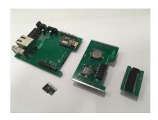
For further diagnostics, connect the OLED board to the CPU board.
