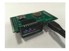
• If the CPU board doesn't start correctly or the Memory Card icon is flashing on the OLED display, proceed with formatting the SD card (see Appendix 1).
