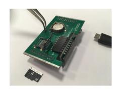
o While keeping the contacts short-circuited, connect the CPU board via a USB cable to your PC with the installed Swift CPS.
