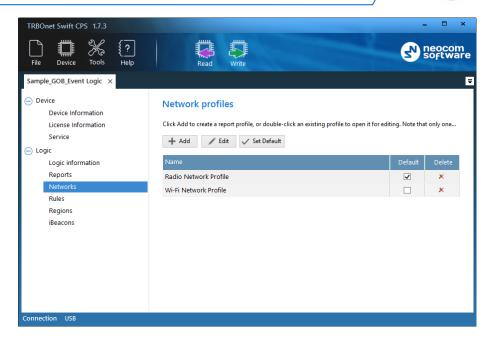
The **Network profiles** tab displays all profiles with network settings that are defined in the opened configuration.
