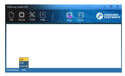
The selected connection appears on the status bar, for example, "Connection: LAN".
