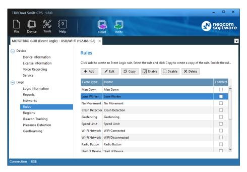
To configure rules, expand the **Logic** section and click **Rules** in the left panel.
