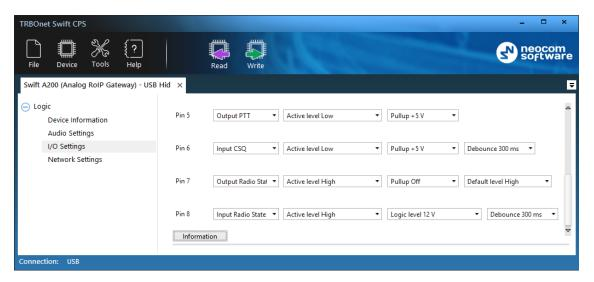
In the right panel, the physical I/O connector pins of Swift A200 appear as labels **Pin 1** through **Pin 8**. For each connected physical pin, specify the settings as described in the following table.
