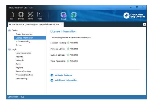
In the right panel, all the licensed features that are supported by your device are marked as **Activated**, **Available for activation**, or **Not available** (not supported on your type of device).
