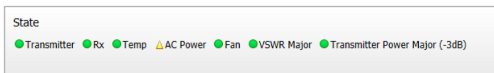
Figure 39: The State panel displays the AC Power alarm with the minor severity level
