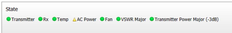
Figure 38: The State panel displays the AC Power alarm with the minor severity level
