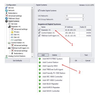
All radio system elements based on MOTOTRBO services are represented in the **Registered Digital Systems** table, including their type (Control Station, Repeater, and others), IP Address, and Radio ID (1):
