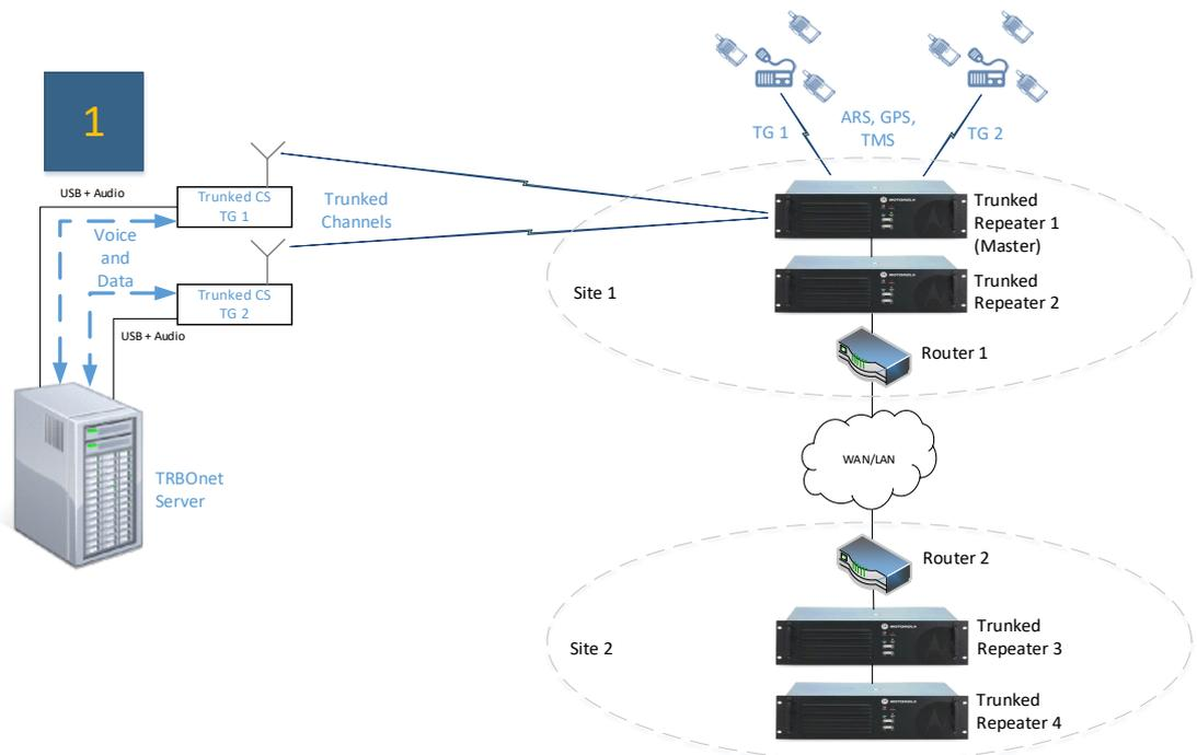
Figure 1: System with Trunked Control Stations
