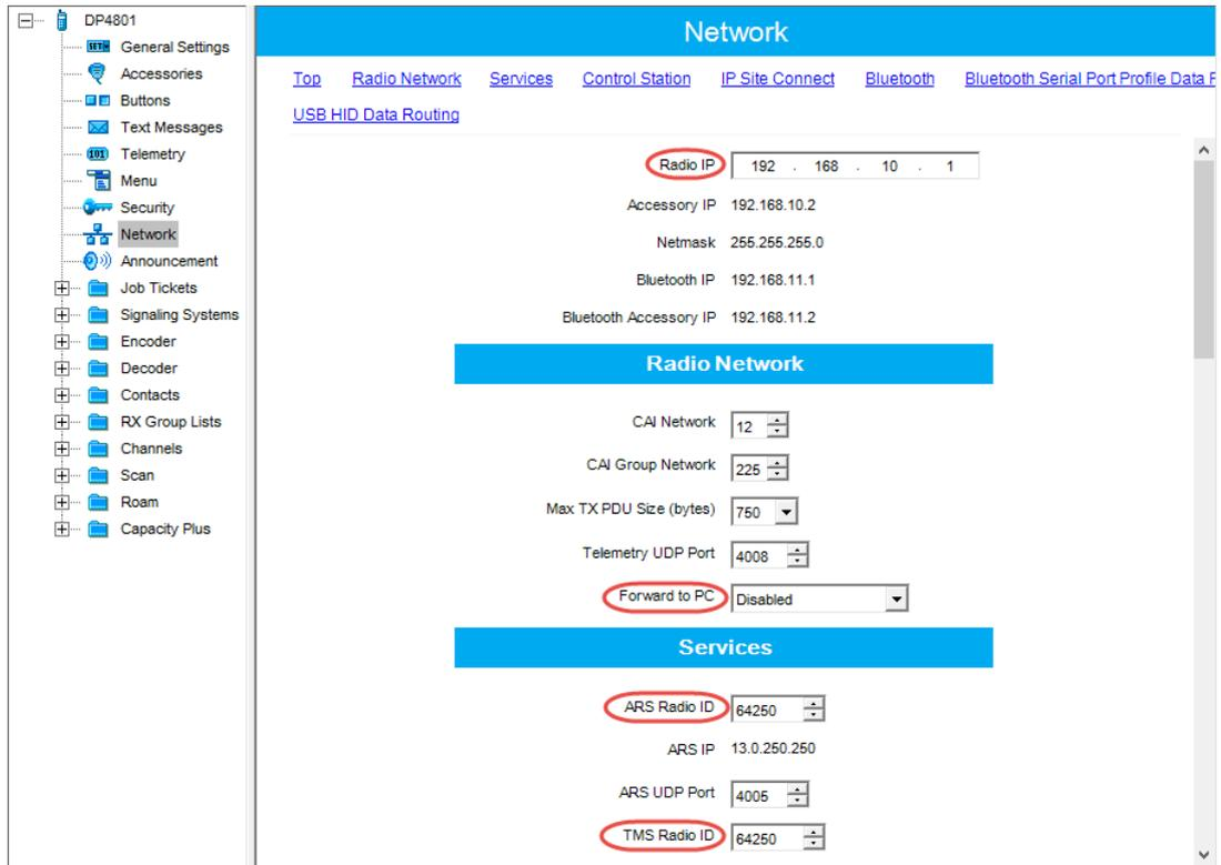
The screenshot displays the configuration page for a device (DP4801) under the 'Network' category. The left sidebar lists various settings, with 'Network' highlighted. The main area shows the 'Radio Network' and 'Services' sections. Key parameters are highlighted with red circles:
