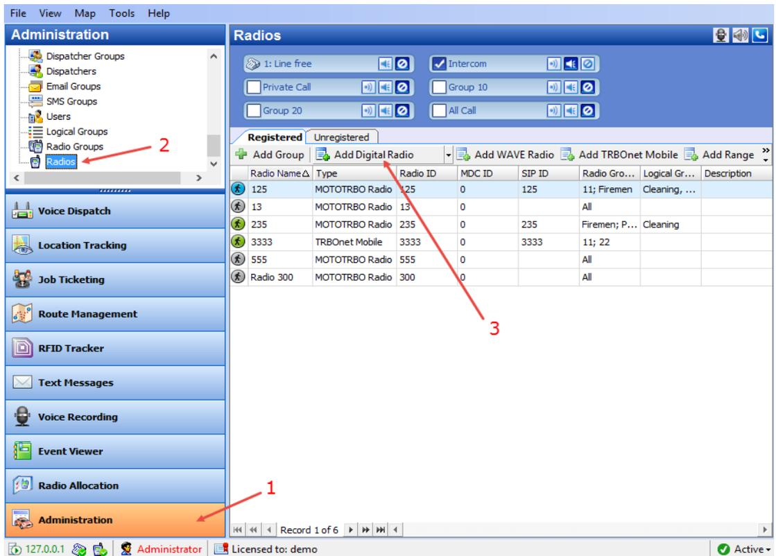
The screenshot shows the Neocom software interface. The left sidebar contains a tree view with 'Administration' highlighted in orange (1). The main window is titled 'Radios' and contains a table of registered radios. The 'Add Digital Radio' button is highlighted with a red arrow (3).
